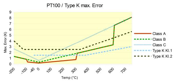
Maximal <u>allowed</u> error for PT resistors class A/B/C and Thermocouple K class 1 and 2.
