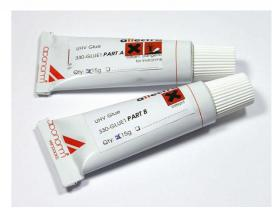
330-GLUE-1 is suitable for high-temperature resistant structural bonding of metals, glass, and ceramics. This adhesive can be used to achieve vacuum tight bonds and it shows remarkably constant adhesive strength even at high temperatures. For the hardening process, a temperature of 130°C is required.
