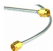
380-SMA18G-MM-300: Ready made RF cable for UHV use. As PTFE must be used for high frequency cables, the cable is not radiation resistant
